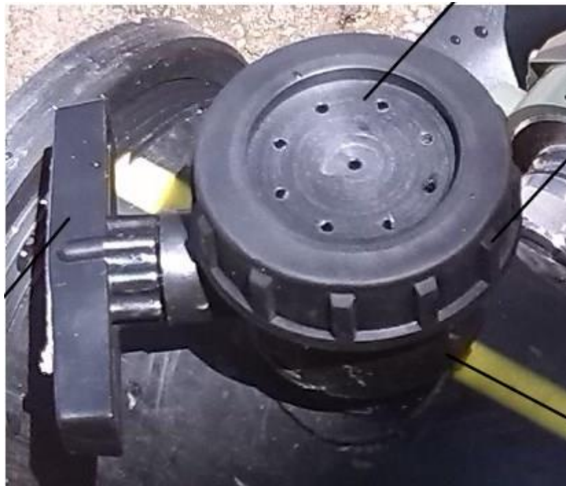
Aeration Nozzle with Butterfly Valve
